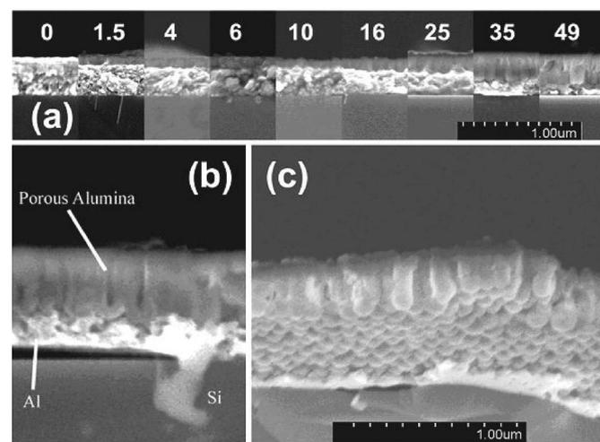
**Figure 3.** (a) Cross-section scanning electron microscopy images of samples anodized for varying times ranging from 1 to 49 s. (b) Magnified image showing pore structure for a sample anodized for 35 s. (c) Scanning electron microscopy images of samples anodized for 49 s under 40 V showing the U-shape bottom that suggest that the relatively short time anodization is sufficient to form a fully developed pore structure.
