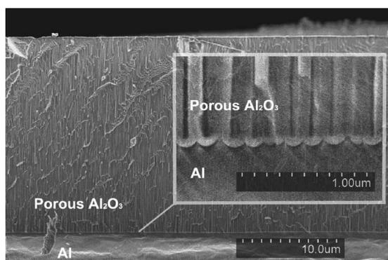
**Figure 6.** Cross-sectional scanning electron microscopy images of samples anodized for 30 min under 60 V and magnified inset images showing the U-shaped barrier layer interface between Al and porous  $\text{Al}_2\text{O}_3$ .
