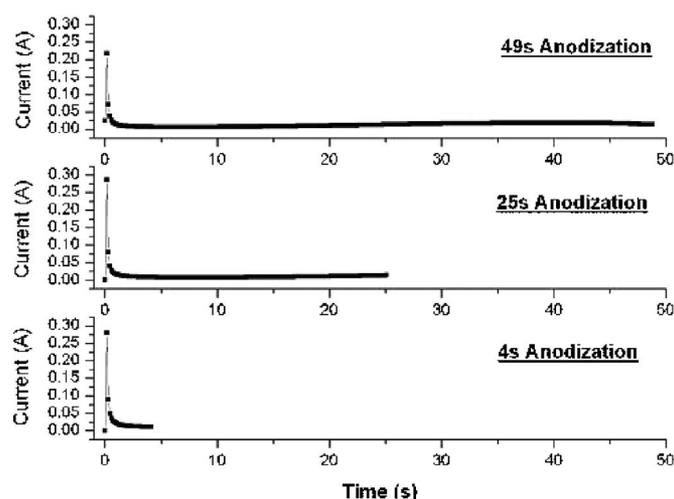
**Figure 2.** Anodization current as a function of time for three representative samples with anodization times 4 s, 25 s, and 49 s.
