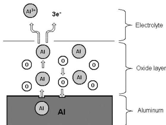
**Figure 1.** A schematic representation of the field-induced counterdiffusion of aluminum and oxygen atoms (or ions). Also indicated is the dissolution of aluminum ions into the electrolyte according to the mechanism of Eq. 3 (i.e., there is no net oxygen dissolution). Oxidation of alumina occurs at the oxide layer–aluminum interface.
