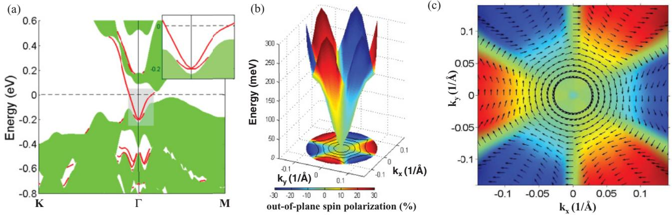
FIG. 1. (Color online) (a) Electronic structure of  $\text{Bi}_2\text{Te}_3$ . Surface states are shown by red (dark gray) lines and projected bulk bands by the green/light gray area. The inset is a blowup of the rectangular light gray area. (b) Energy dependence of  $\text{Bi}_2\text{Te}_3$  surface Dirac cone showing hexagonal warping. Magnitude of out-of-the-plane spin component is indicated by the color bar. (c) In-plane direction of spin on the surface Dirac cone.
