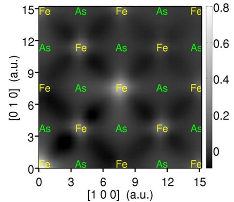
FIG. 3. (Color online)  $\Delta B|_{x_1}^{x_2}(x, y)$  for  $x_2=0.15$  and  $x_1=0.10$ . The yellow labels Fe indicate the atoms in the iron sublattice; green labels As indicate the  $(x, y)$  projection of the atoms in the arsenic sublattice. Atomic assignments are based on the assumption that Fe is at the origin.
