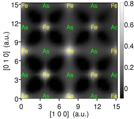
FIG. 4. (Color online)  $\Delta B_{x_1}^{x_2}(x, y)$  for  $x_2=0.15$  and  $x_1=0.10$ , after artificially removing all the Bloch states around  $M$ . Atomic assignments are based on the assumption that Fe is at the origin.
