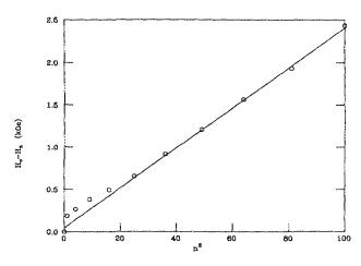
FIG. 2. Field separation of the *n*th spin-wave resonance  $(H_n)$  relative to the main line resonance  $(H_0)$  is plotted vs  $n^2$  for the 3130-Å-thick (001) Fe/ZnSe film.
