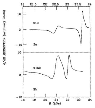
FIG. 3. Absorption derivative vs external applied field data is shown for (a) 840-Å (001) Co/ZnSe and (b) 1070-Å (110) Co/ZnSe films on GaAs substrates.
