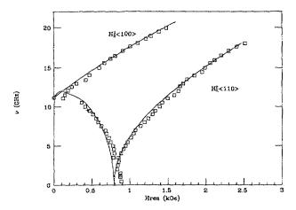
FIG. 1. Frequency vs resonant field dispersion is shown for H collinear to the (100) and (110) axis of the (001) Co/ZnSe film. ( $\square$ ) Slot-line FMR; (+) 9.5 GHz cavity FMR; and (O) zero-field resonance results.
