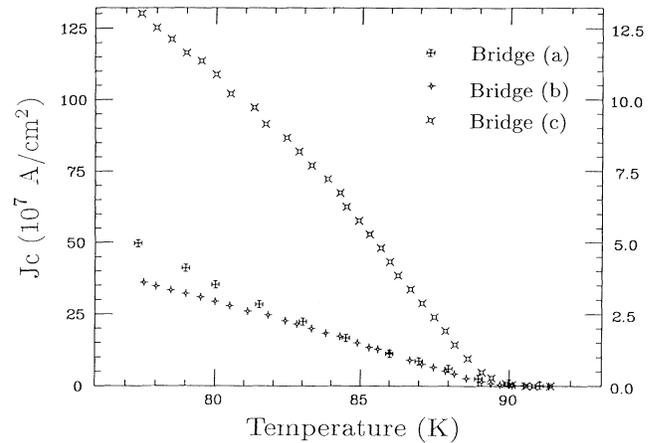
FIG. 3. Critical current densities as a function of  $T$  for the three microbridges. The reader is referred to the scale on the right-hand side of the figure for microbridge (a).
