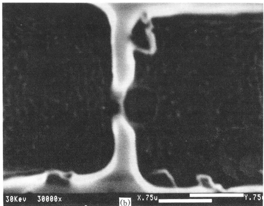
FIG. 1. Geometrical view of two YBCO microbridges.  $L = 4000 \text{ \AA}$  for bridge (a) and  $L = 500 \text{ \AA}$  for bridge (b). The bright area is YBCO film and the black is substrate.
