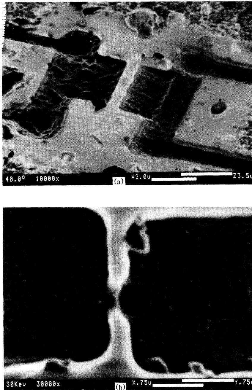
FIG. 1. Geometrical view of two YBCO microbridges.  $L = 4000 \text{ \AA}$  for bridge (a) and  $L = 500 \text{ \AA}$  for bridge (b). The bright area is YBCO film and the black is substrate.
