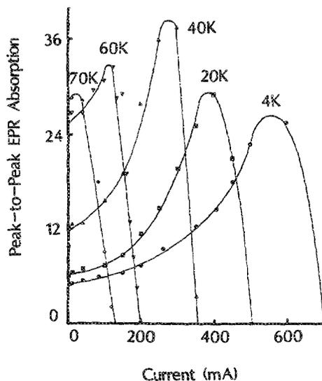
FIG. 2. Peak-to-peak values of the differential microwave absorption signals measured as function of current at various temperatures.
