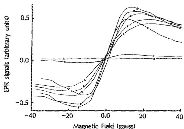
FIG. 1. Differential EPR signals for various imposed currents at  $T = 40 \text{ K}$ .
