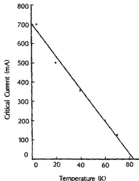
FIG. 4. Plot of critical current vs temperature.
