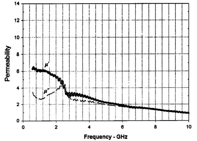
FIG. 7. Zero-field permeability data for oriented Y-type hexaferrite from 0 to 10 GHz.
