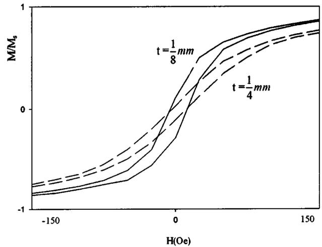
FIG. 4. Normalized magnetization is plotted as a function of external field. The parameter  $t$  is the slab thickness (solid line:  $t=0.125$  mm, dashed line:  $t=0.25$  mm) and  $4\pi M_s$  is the saturation magnetization.
