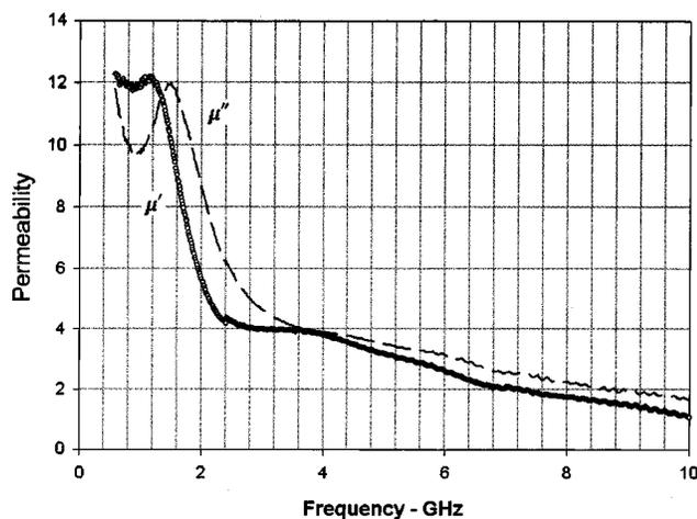
FIG. 3. Zero-field permeability data for single crystal Y-type hexaferrite from 0 to 10 GHz.
