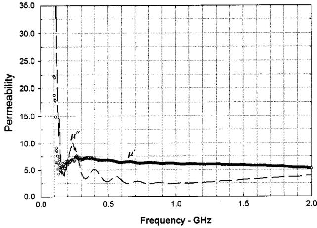
FIG. 6. Zero-field permeability data for oriented Y-type hexaferrite from 0 to 2 GHz.
