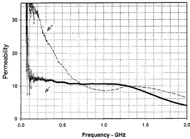
FIG. 2. Zero-field permeability data for single crystal Y-type hexaferrite from 0 to 2 GHz.
