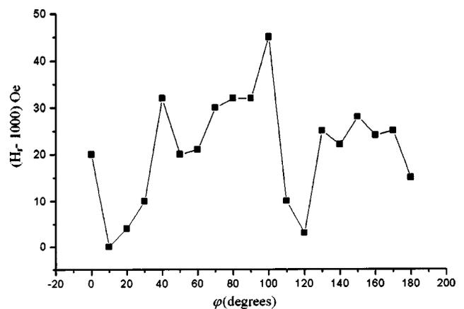
FIG. 5. In-plane FMR at 9.56 GHz,  $\phi$  is the in-plane angle of rotation.
