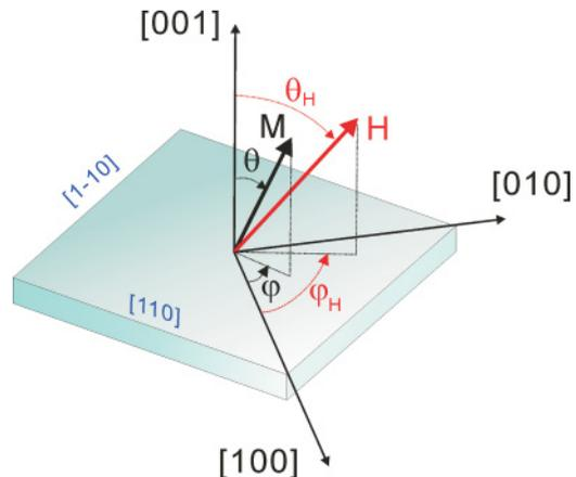
FIG. 1. (Color online) Coordinate system used in this work that describes the orientation of the dc magnetic field  $H$  and resulting equilibrium orientation of the magnetization  $M$  with respect to the crystallographic orientation of the  $\text{Co}_2\text{MnSb}$  films.
