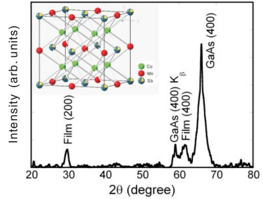
FIG. 3. (Color online) XRD spectrum of  $\text{Co}_2\text{MnSb}$  film. Inset illustrates an  $L2_1$ -type structure.
