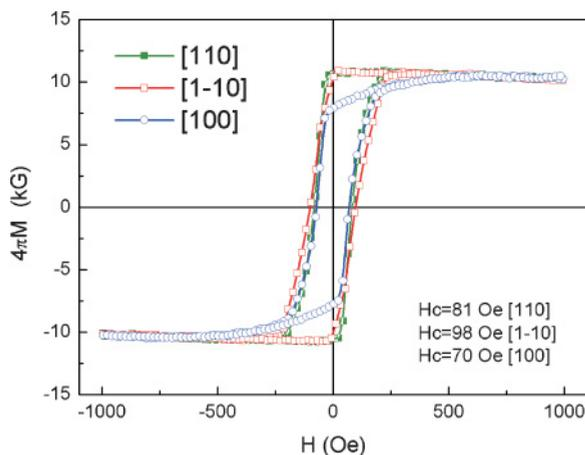
FIG. 5. (Color online) Magnetic hysteresis loops of  $\text{Co}_2\text{MnSb}$  film magnetized along different crystal axes. The diamagnetic slope in each curve originates from the GaAs substrates (see text).
