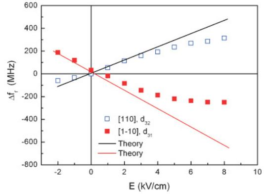
FIG. 9. (Color online) Variation of FMR frequency with applied electric-field strength for the Co<sub>2</sub>MnSb/GaAs/PZN-PT heterostructure. Solid and hollow symbols denote the measured values, whereas the solid lines represent the theoretical prediction.
