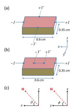
FIG. 1. (Color online) Schematics of transport measurements. (a) Magneto-electric resistance  $R_{xy}(\mathbf{H})$ . (b) Magnetoresistance  $R_{xx}(\mathbf{H})$ . (c) Direction of applied magnetic field,  $0 \le \theta \le 90$  and  $0 \le \phi \le 90$ .
