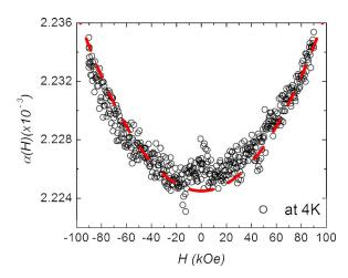
FIG. 3. (Color online) Magnetoelectric coefficient,  $\alpha(\mathbf{H})$  (symbols), data from magnetoelectric conductivity. Dashed line shows fitting experimental ME coefficient with equation shown in Eq. (8).
