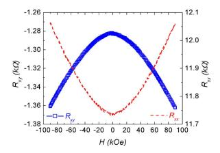
FIG. 2. (Color online) Magnetoresistance  $R_{xx}(\mathbf{H})$  (dashed line) and magnetoelectric resistance  $R_{xy}(\mathbf{H})$  (solid symbols) measured in function of magnetic field at temperature T=4 K.
