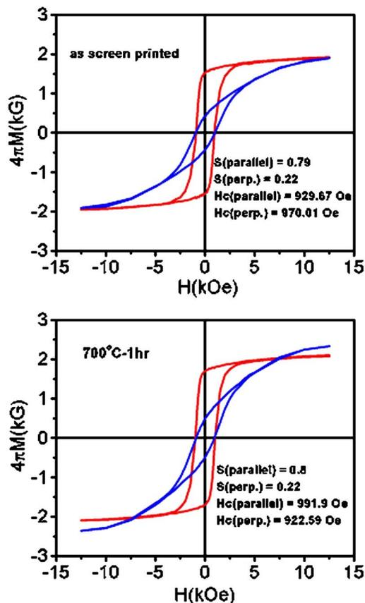
FIG. 3. (Color online) The hysteresis loops of the  $\text{BaFe}_{11.2}\text{Sc}_{0.8}\text{O}_{19}$  after annealing at  $700^\circ\text{C}$  for 1 h. The inequivalency in the in-plane measurement near the maximum field is related to the pole gap.
