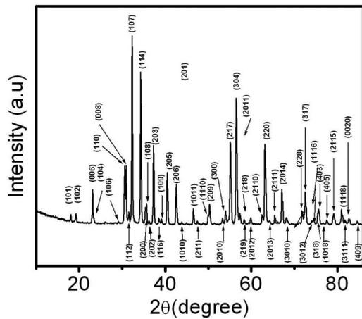
FIG. 1. X-ray diffractogram of representative  $\text{BaFe}_{11.2}\text{Sc}_{0.8}\text{O}_{19}$  powder sample.
