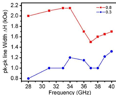
FIG. 4. (Color online) FMR linewidth ( $\Delta H$ ) vs frequency for the in-plane oriented, screen printed annealed  $\text{BaFe}_{11.7}\text{Sc}_{0.3}\text{O}_{19}$  and  $\text{BaFe}_{11.2}\text{Sc}_{0.8}\text{O}_{19}$  films.
