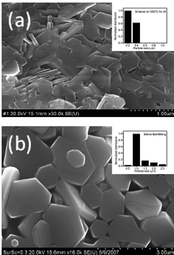
FIG. 2. Scanning electron micrographs of  $\text{BaFe}_{11.7}\text{Sc}_{0.3}\text{O}_{19}$  sintered at (a) 1000 °C for 2 h, (b) 1150 °C for 2 h, (b) the insets of the figures show the particle size distribution.
