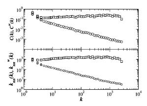
FIG. 13. N=5000;  $s_0=10^4$ . Correlations and clustering for a=0.6,  $\delta=0.1$ . Unweighted quantities  $[k_{nn}(k)]$  and C(k) are shown by circles, weighted quantities  $[k_{nn}^w(k)]$  and  $C^w(k)$  by squares.
