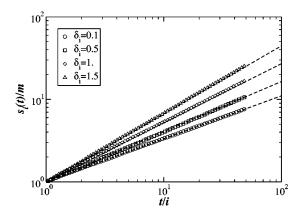
FIG. 7. Model with random  $\delta_i$ : evolution of  $s_i/m$  for a given node i with various values of its redistribution parameter  $\delta_i$ . m=2,  $N=10^4$ , average over 1000 networks with the same realization of  $\delta_j \in [0;2]$   $(j \neq i)$ . The dashed lines correspond to the predicted power laws  $(t/i)^{a(\delta_i)}$ .
