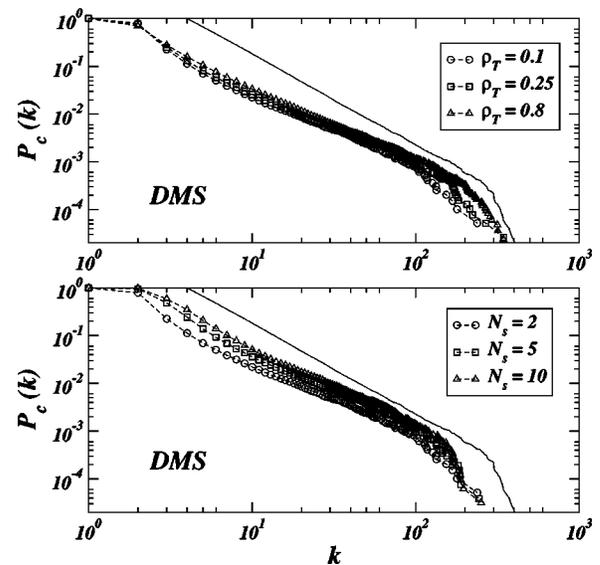
FIG. 6. Cumulative degree distribution of the sampled DMS graph for USP probes. The top figure shows sampled distributions obtained with  $N_S=2$  and varying density target  $\rho_T$ . The figure on the bottom shows sampled distributions obtained with  $\rho_T=0.1$  and varying number of sources  $N_S$ . The solid line is the degree distribution of the underlying graph.
