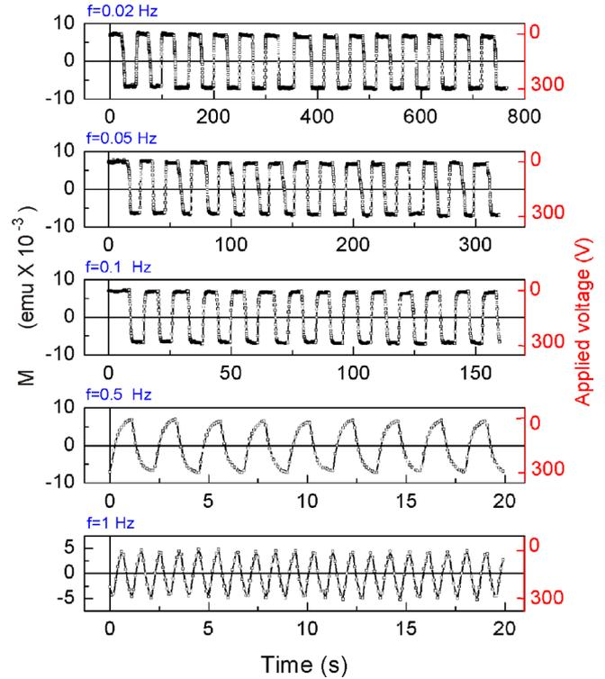
FIG. 2. (Color online) Magnetization switching under application of a square waveform electric field at different frequencies.
