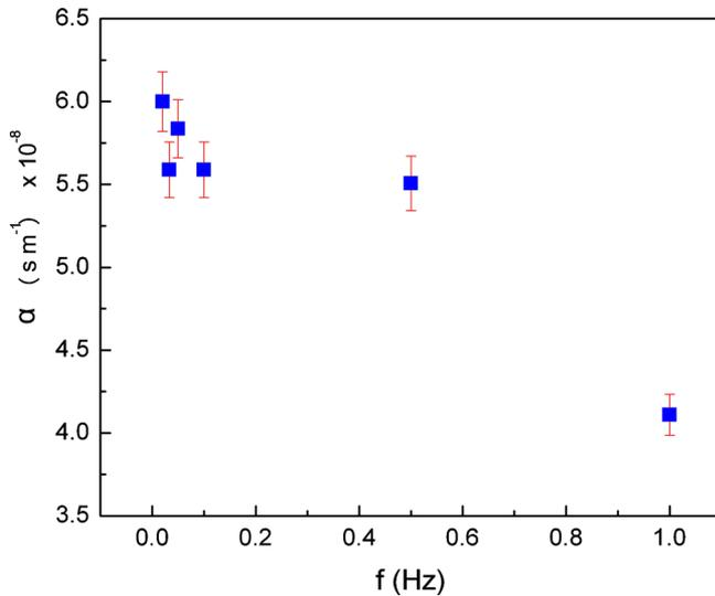
FIG. 3. (Color online) Frequency dependence of the converse magnetoelectric coupling coefficient in a FeCoV/PMN-PT heterostructure.
