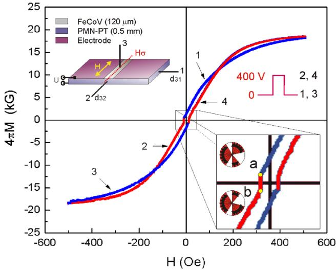
FIG. 1. (Color online) Magnetic hysteresis loop controlled by an applied electric voltage for an FeCoV/PMN-PT heterostructure. Upper left inset: Sketch of field configuration and geometries of the heterostructure. Right lower inset: Enlargement of the magnetization switched by an electric field and spin configurations in two magnetization states.
