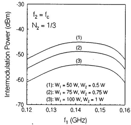
FIG. 2. Calculated intermodulation power output for  $f_2=2f_c-f_1$  and  $N_z=1/3$ .
