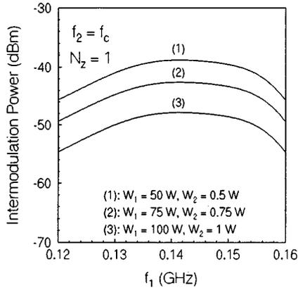
FIG. 1. Calculated intermodulation power output for  $f_2=2f_c-f_1$  and  $N_z=1$ .
