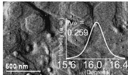
FIG. 1. AFM micrograph of the barium hexaferrite thin film. Rocking curve measurement of the  $\langle 008 \rangle$  barium hexaferrite peak (inset).
