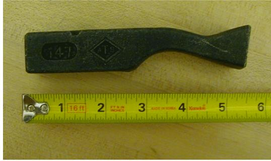
Figure 3: Hand Held Bucking Bar
