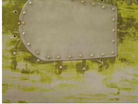
Figure 5: Repair patch on airplane fuselage
