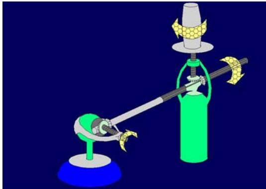
Figure 9 – Mechanical Articulating Arm: The mechanical arm design is overly complex with too many moving parts.
