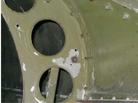
Figure 8 – Interior of an Airplane Fuselage: This is an example of possible obstacles and curved surfaces that the riveting helper device might encounter. The positioning system must be able to hold the bucking bar assembly perpendicular to the sheet metal surface.
