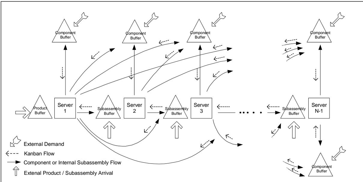
**Figure 2. Kanbans and Materials Flows in a Disassembly Line**
