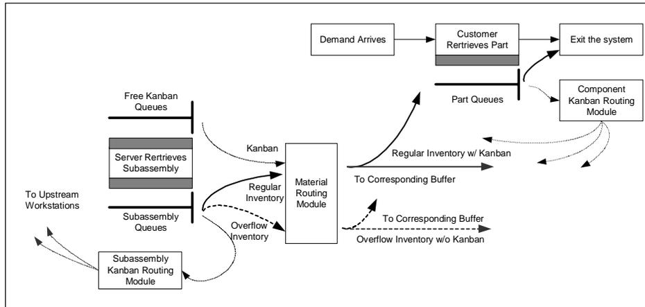
**Figure 3. The Multi-Kanban Mechanism**
