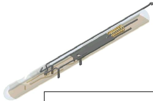
Figure 4.9b: Pull-pull receptor system
