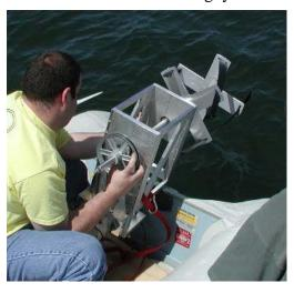
Figure G.2: Hydroelectric Power Generator Attached to Dinghy
