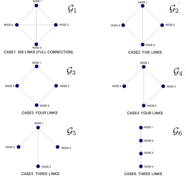
Fig. 2. Six different configurations of topology.
