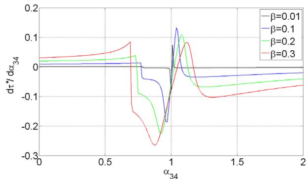
Fig. 10. Damping effect to sensitivity of delay margin as  $\alpha_{34}$  changes in  $\mathcal{G}_2$ .
