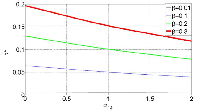
Fig. 12. Damping effects to delay margin as  $\alpha_{14}$  changes in  $\mathcal{G}_3$ .
