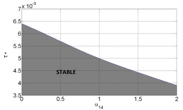
Fig. 6. Delay margin  $\tau^*$  with respect to  $\alpha_{14}$  in  $\mathcal{G}_3$ . Shaded region corresponds to stable dynamics.  $\beta = 0.01$ .
