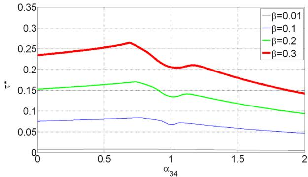
Fig. 9. Damping effect to delay margin as  $\alpha_{34}$  changes in  $\mathcal{G}_2$ .
