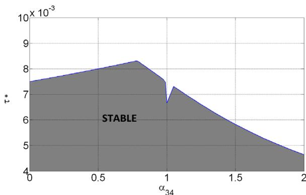
Fig. 4. Delay margin  $\tau^*$  with respect to  $\alpha_{34}$  in  $\mathcal{G}_2$ . Shaded region corresponds to stable dynamics.  $\beta = 0.01$ .
