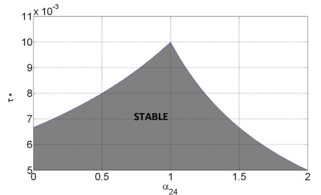
Fig. 7. Delay margin  $\tau^*$  with respect to  $\alpha_{24}$  in  $\mathcal{G}_1$ . Shaded region corresponds to stable dynamics.  $\beta = 0.01$ .
