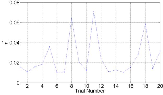
Fig. 8. Stability margin of the system with the topology  $\mathcal{G}_1$  for 20 different trials, where in each trial all the six coupling strengths  $\alpha_{\mu k}$  are randomized from a uniform distribution with  $\alpha_{\mu k}$  being between zero and one, and where each randomization is seeded with the computer clock.
