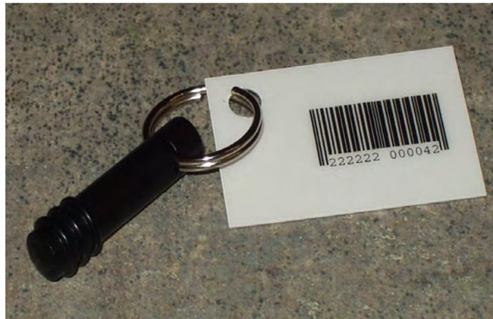
*Figure 12. RI-TRP-WFOB-01 LF RFID tag and barcode label*
