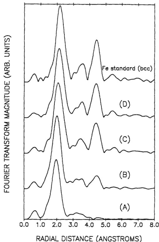
Figure 3. Fourier transforms of conversion-electron EXAFS spectra of specimens in the as-deposited and magnetic field annealed states. The Fourier transform of the Fe standard is included for
