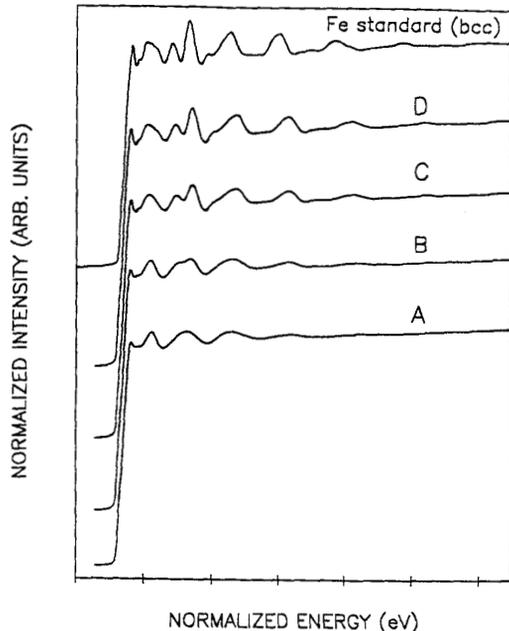
Figure 2. Conversion-electron x-ray absorption fine structure spectra for as-deposited and annealed specimens of amorphous IBS Co<sub>74</sub>-Fe<sub>6</sub>-B<sub>15</sub>-Si<sub>5</sub> (specimens A,B,C,D) and for IBS Fe film.
