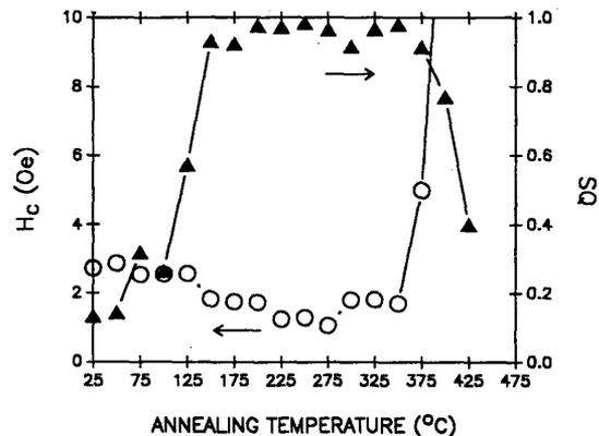
Figure 1. Variation of film coercive field ( $H_c$ ) and hysteresis loop squareness (SQ) with annealing temperature for an IBS  $\text{Co}_{74}\text{Fe}_6\text{B}_{15}\text{Si}_5$  film ( $t=150$  nm). Data was extracted from hysteresis loops acquired at annealing temperatures (annealing time approx. 16 min.) via VSM.
