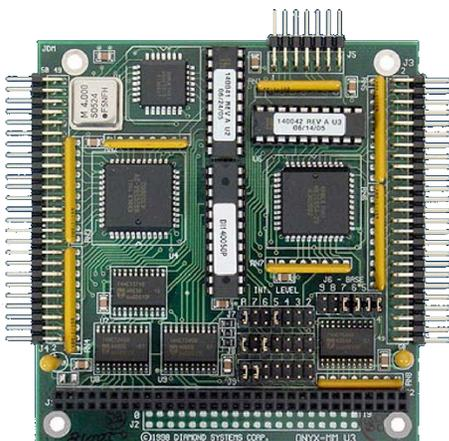
Figure 5 - Digitally Controlled I/O Module
