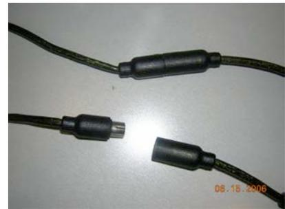
**Figure 10 - Quick Connect from Xbox controller**
