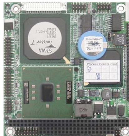
Figure 6 - PC/104 Embedded CPU
