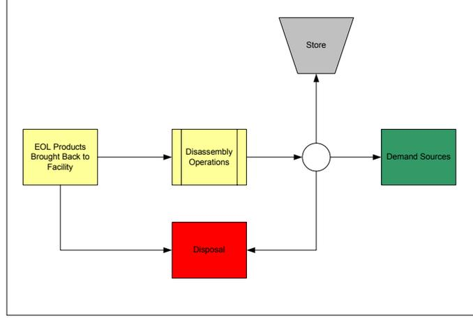
Figure 2. Process flow in disassembly facility
