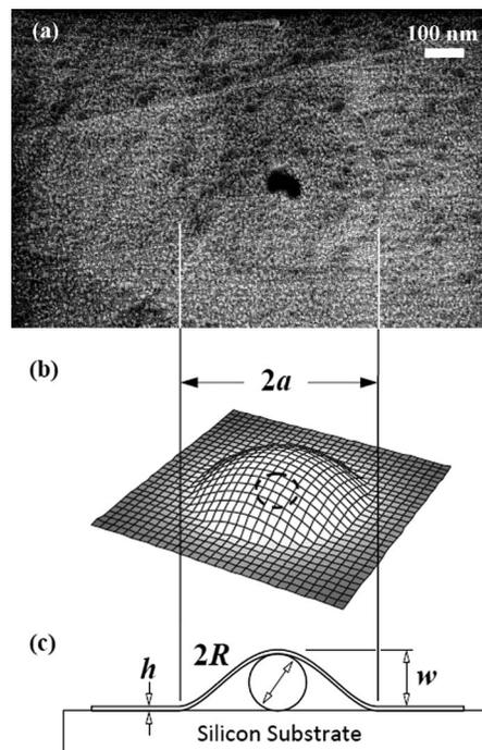
FIG. 2. A typical circular blister trapping two nanoparticles at the interface. (a) A SEM image. The contrast is inverted to highlight the blister periphery so the two trapped particles appear dark (scale bar=100 nm). (b) A 3D representation. (c) Sketch of blister for theoretical modeling.
