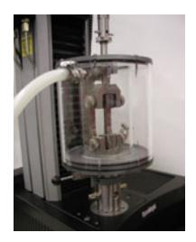
Figure 3: Instron Biopulse Device
