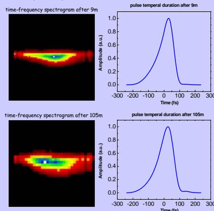
Fig. 5. Pulse time-frequency spectrogram and pulse duration after 9m and 105m propagation in the air.
