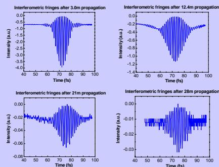
Fig. 3 Pulse interferometric fringes after different propagation distances
