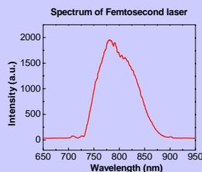
Fig. 2 Spectrum of 10 femtoseconds laser pulse. The central wavelength is 798nm, The HMFWM is 99nm.
