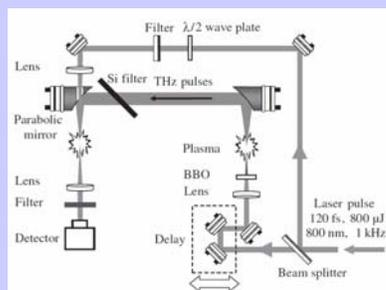
Fig. 1 Schematics of experimental setup for THz wave generation and detection in air
