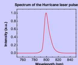
Fig. 4 Spectrum of Hurricane femtosecond laser. The central wavelength is 798nm, The HMFWM is 9nm.
