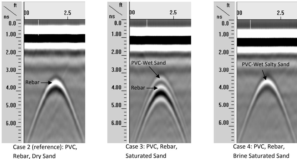
Figure 4.3: B-scan results for test cases 2, 3, and 4
