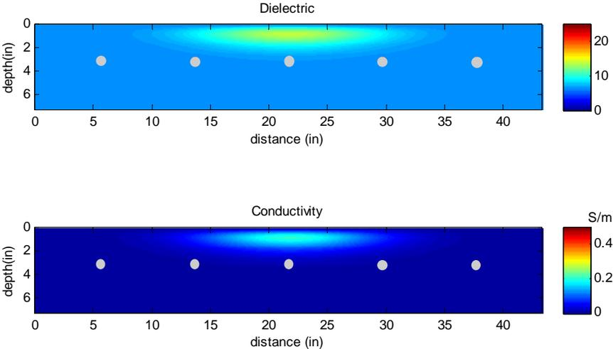
**Figure 4.8: Mapping of dielectric and conductivity for Model 2 with contamination concentrated under the surface (rebar in gray)**
