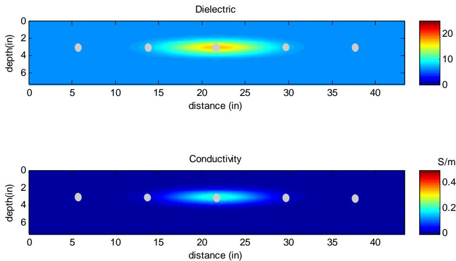
**Figure 4.5: Mapping of dielectric and conductivity for Model 1 with contamination extending from rebar (gray)**
