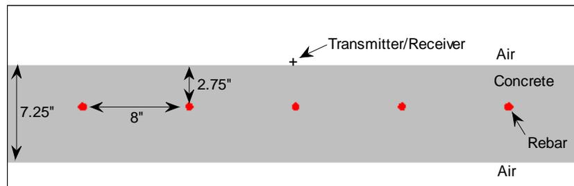
Figure 4.4: Bridge Deck Modeled with the ISSME software
