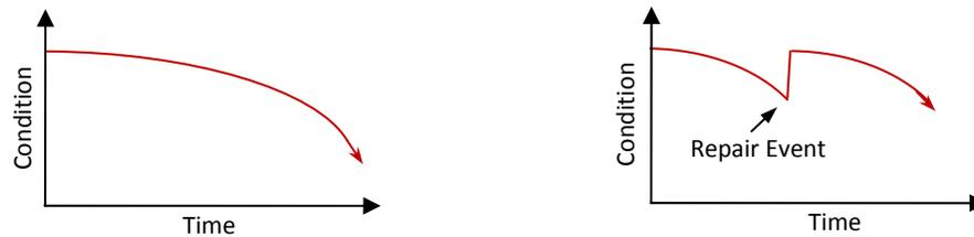
**Figure 1.1: Illustrative models for deterioration of bridge decks over time**
