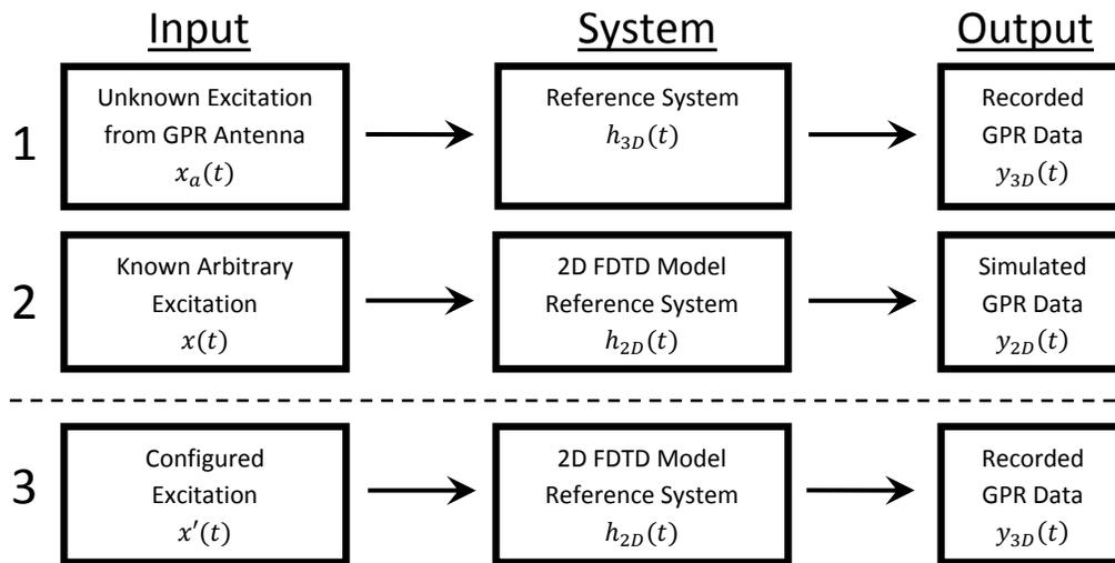
Figure 3.1: Diagram of the three input-system-output relationships used to configure the FDTD excitation
