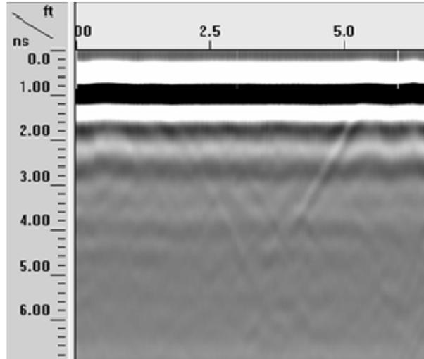
Figure 4.2: Case 1: B-scan of soil bed with PVC filled with dry sand shows no indication of the buried target
