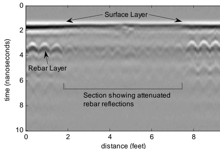
**Figure 2.6: B-scan showing a potentially deteriorated section of bridge deck (data courtesy of Ken Maser, Infrasense, Inc.)**
