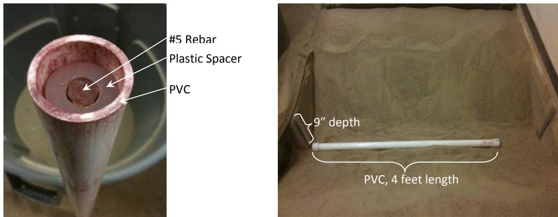
**Figure 4.1:** *Left:* Experimental setup with PVC, spacer, and rebar. *Right:* PVC placed in soil bed prior to burying
