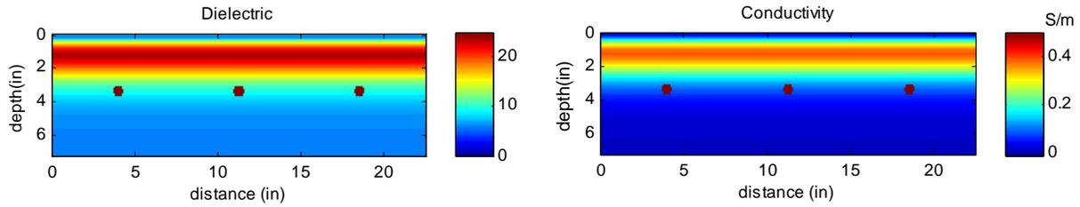
**Figure 4.14: Material model for contaminated concrete with parameters calculated from GPR bridge deck data**
