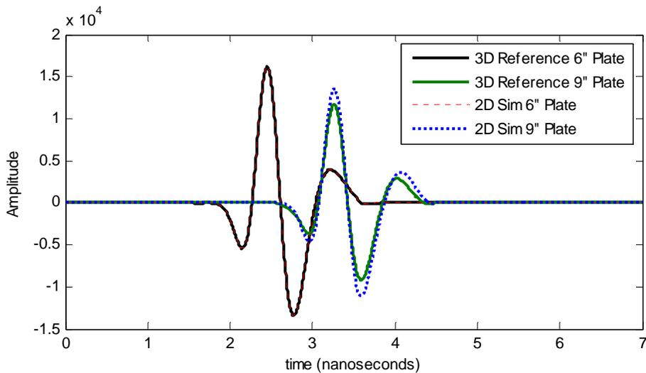
Figure 3.4: Comparison of 3D reference scans and 2D simulated scans using  $x'_6(t)$  as an excitation signal.
