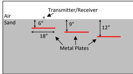
**Figure 3.2: Left: Burying the deepest of 3 metal plates for the reference system. Right: 2D FDTD model of the reference system**
