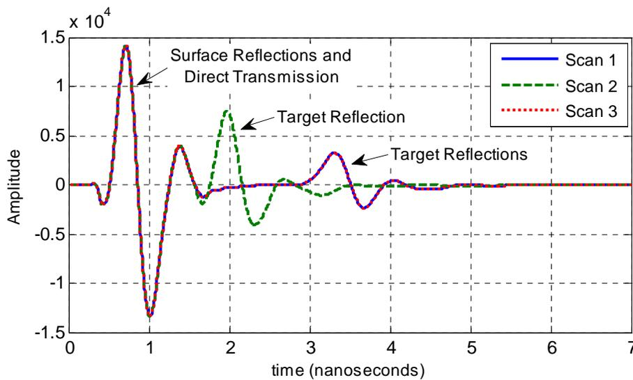
Figure 2.4: Scans recorded at the three antenna positions shown in Figure 2.3
