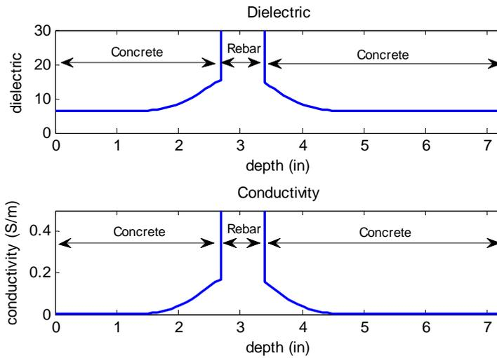
**Figure 4.6: Profiles of material properties through the center rebar for Model 1**
