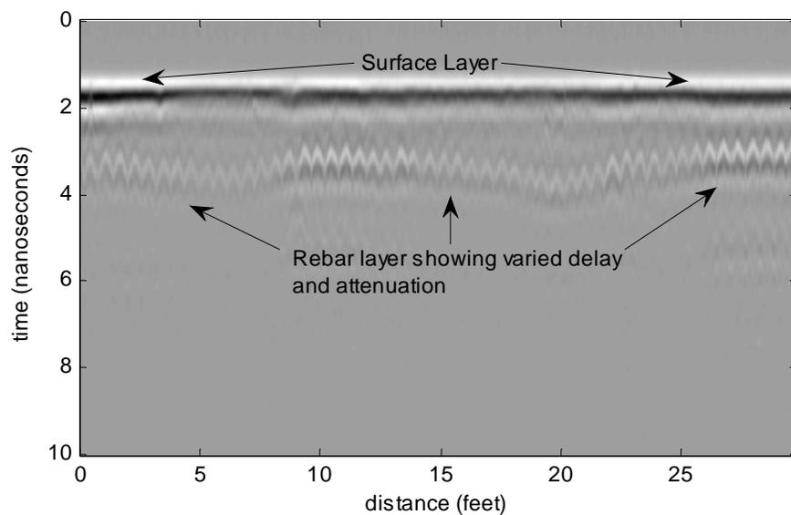
Figure 2.7: B-scan showing rebar layer with obvious variations (data courtesy of Ken Maser, Infrasense, Inc.)
