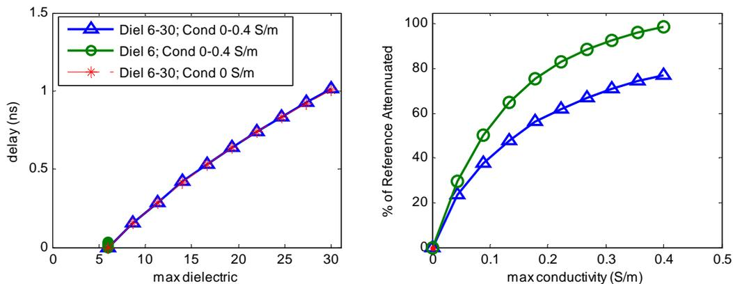
**Figure 4.11: Left: Delay of the rebar reflection vs. the maximum dielectric constant in the material model. Right: Attenuation of the rebar reflection vs. the maximum conductivity in the material model**
