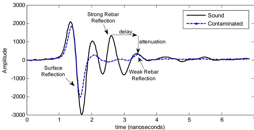
**Figure 4.13: Comparison of center rebar scans where in contaminated concrete the rebar reflection is delayed and attenuated compared to the rebar reflection in sound concrete**
