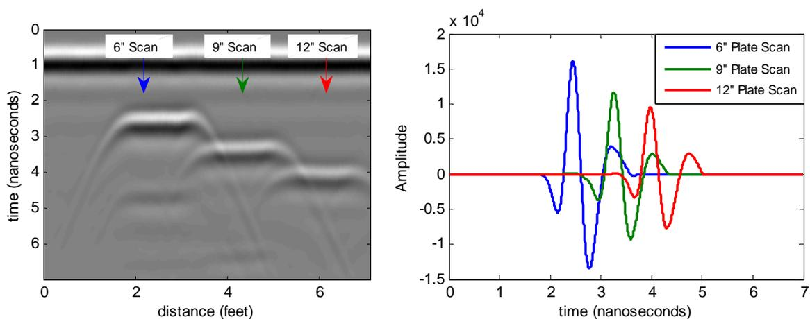
**Figure 3.3: Left: B-scan showing reflections from 3 metal plates and locations of scans (time histories) for each plate. Right:**
