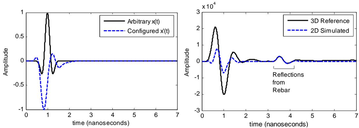
**Figure 3.6: Left: Normalized excitations used with the 2D FDTD model. Right: Comparison of reference case GPR data to simulated response using the configured excitation**
