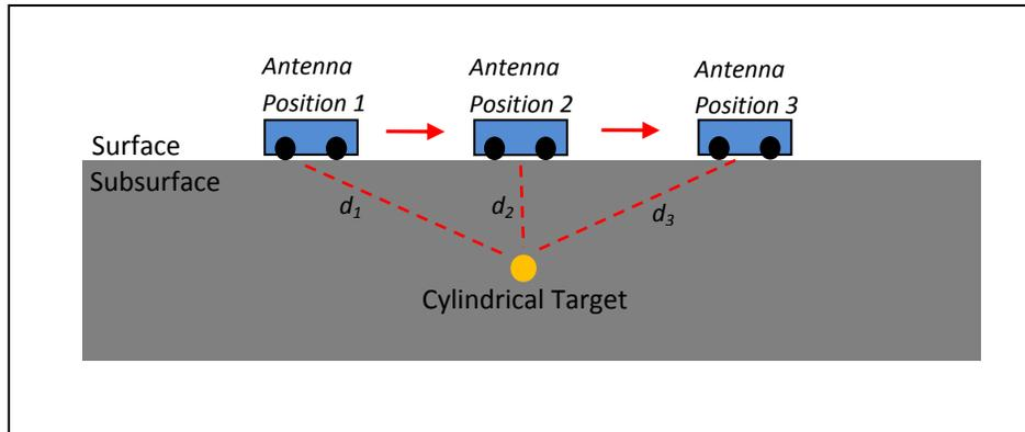
Figure 2.3: Three positions of a GPR antenna as it crosses a cylindrical target
