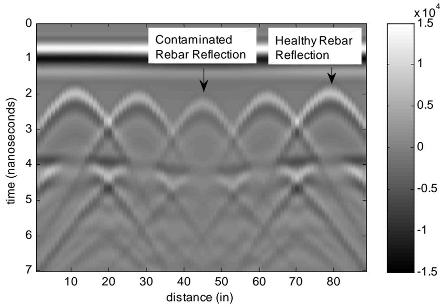
**Figure 4.10: Simulated B-scan of Model 2 showing delay and attenuation of the rebar reflection in the contaminated area**
