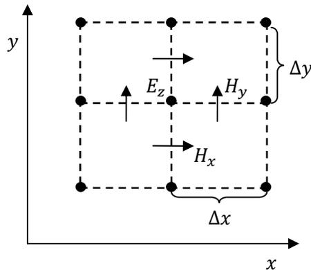
Figure 2.8: Arrangement of the electric and magnetic fields used in Equation 2.7
