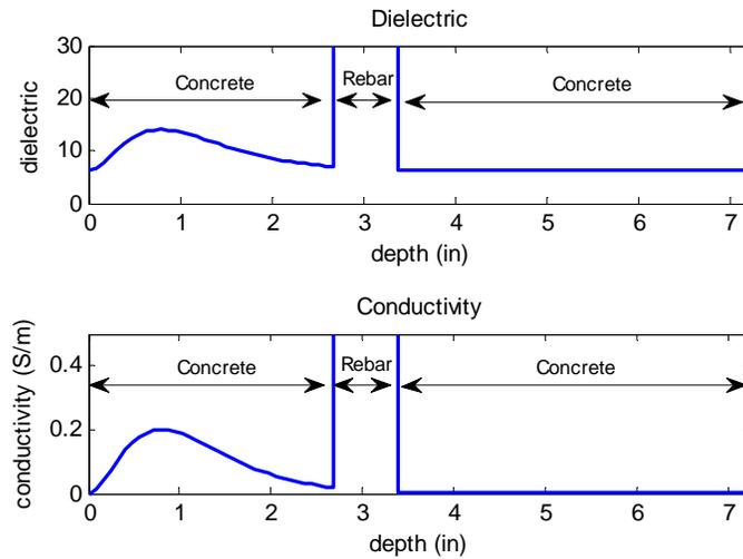
**Figure 4.9: Profile of material properties through the center rebar in Model 2**
