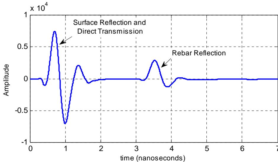
**Figure 2.2: Typical scan, or time history of reflection amplitude, recorded by GPR over a reinforcing bar**
