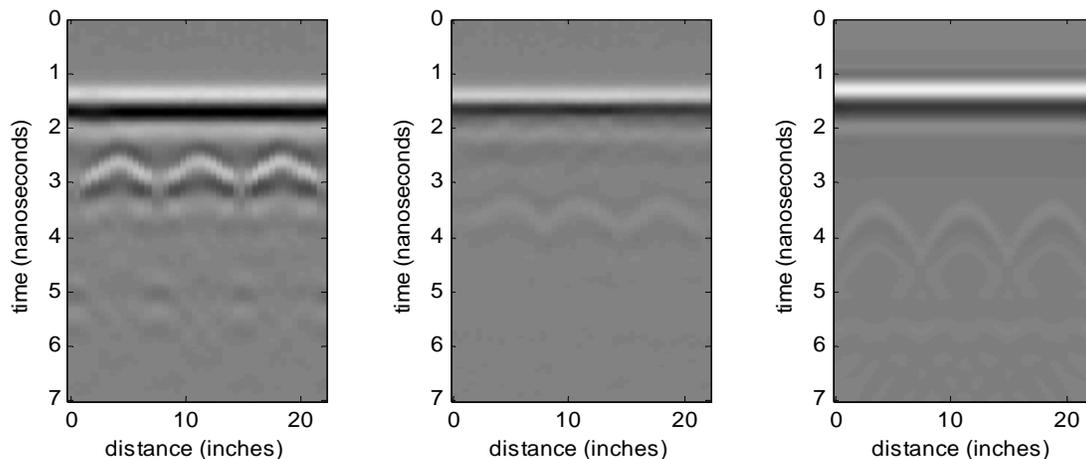
**Figure 4.12: Left: Reference GPR data. Center: Contaminated GPR data. Right: Simulated B-scan using material Model 2 and calculated parameters (GPR data courtesy of Ken Maser, Infrasense)**
