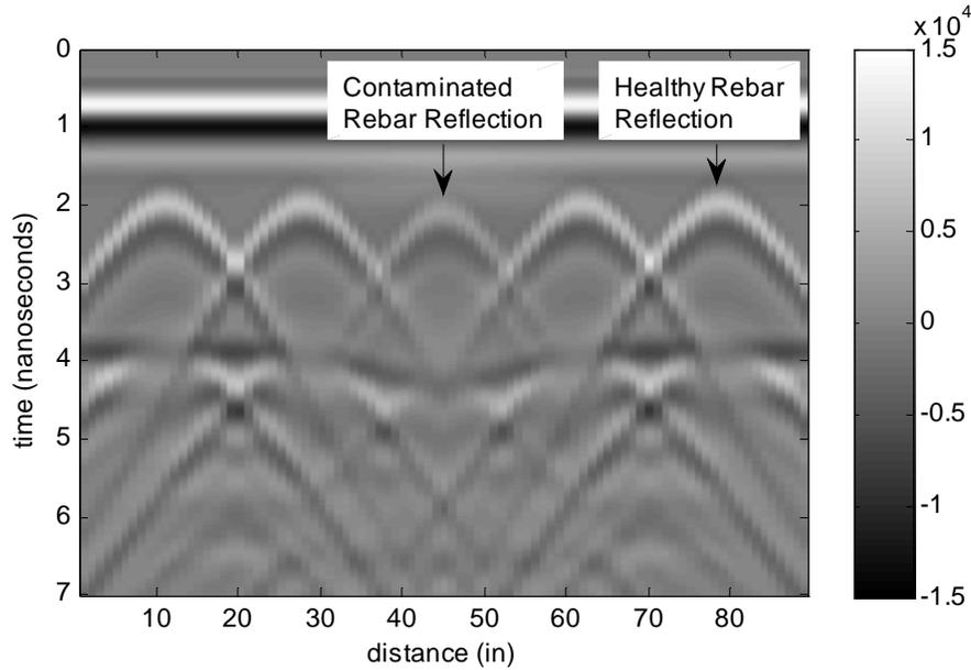
**Figure 4.7: Simulated B-scan of Model 1 showing delay and attenuation of the rebar reflection in the contaminated area**
