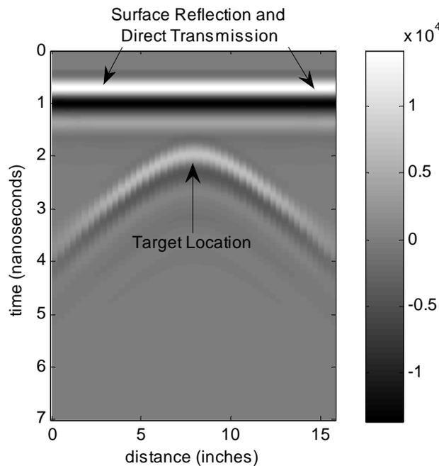
Figure 2.5: B-scan collected over a cylindrical metal target
