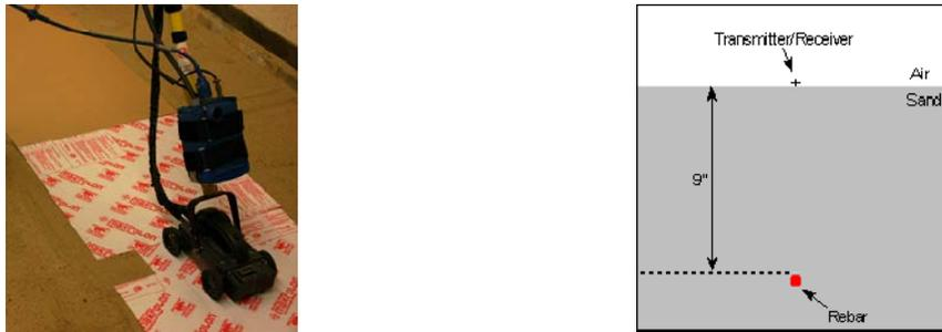
Figure 3.5: *Left:* Collecting GPR data for the reference case. *Right:* 2D FDTD model of the reference case
