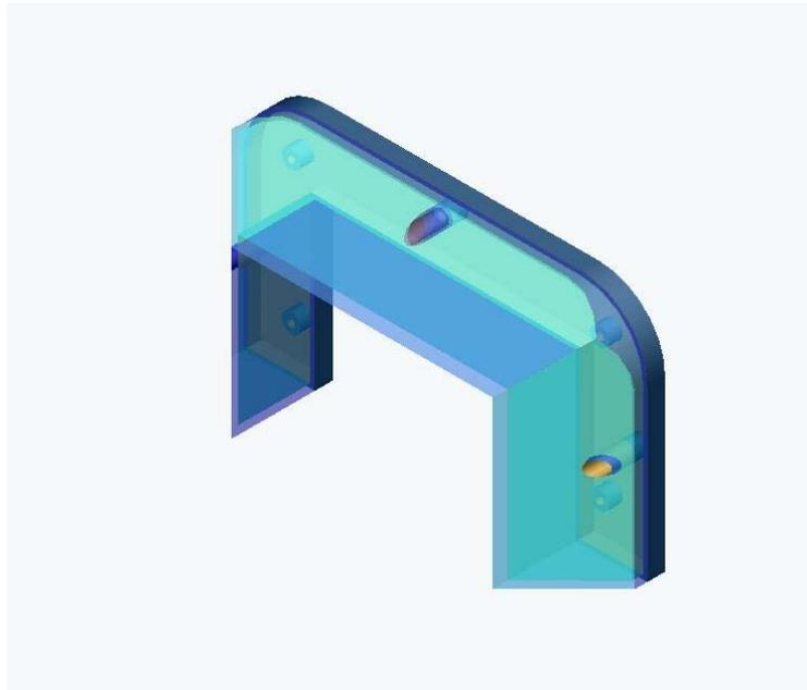
**Figure 4.6 – Two piece light housing**
