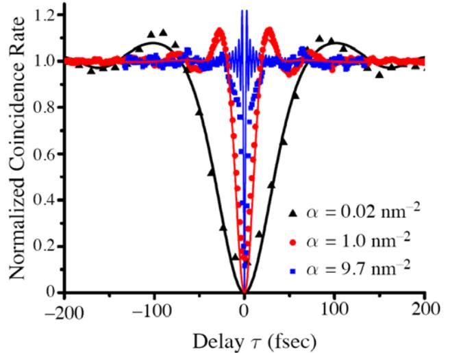
**Figure 3. Normalized Hong-Ou-Mandel (HOM) coincidence interferograms (dips) for various values of the chirp coefficient  $\alpha$ . The symbols represent the measured data points whereas the solid curves are the corresponding numerical simulations. The FWHM of the measured dips are 77, 19.1, and 7.16 fsec for three values of the chirp parameter  $\alpha$ .**
