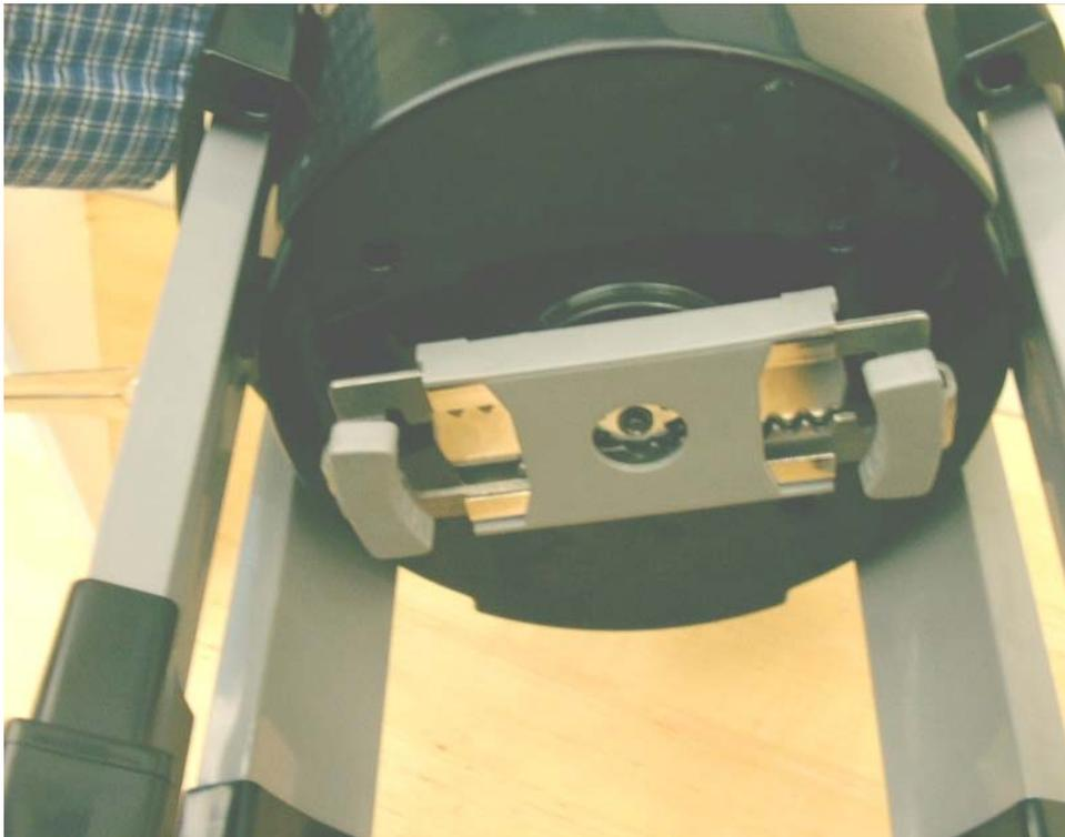
Figure 6.4 – Top platform gear track
