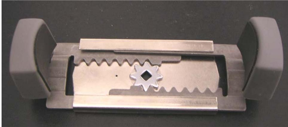
Figure 6.5 – Base gear track after disassembly
