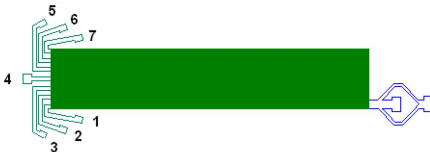
**Figure 14: Final device design consisted of a longer separation zone to maximize the area available for cell movement**
