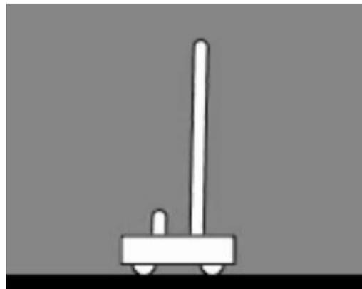
*Figure 4: Depiction of double cart-pole balancing*
