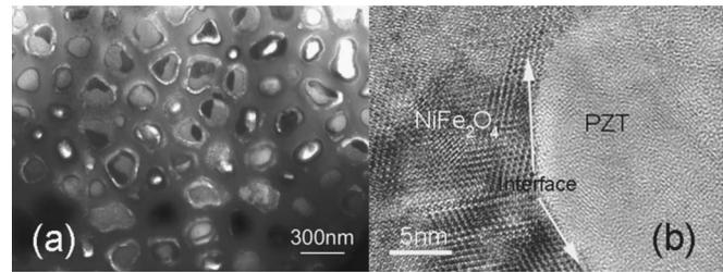
FIG. 4. (a) Cross-section TEM image of core-shell PZT- $\text{NiFe}_2\text{O}_4$  nanowire in AAO template and (b) cross-section HRTEM image of core-shell PZT- $\text{NiFe}_2\text{O}_4$  interface area.
