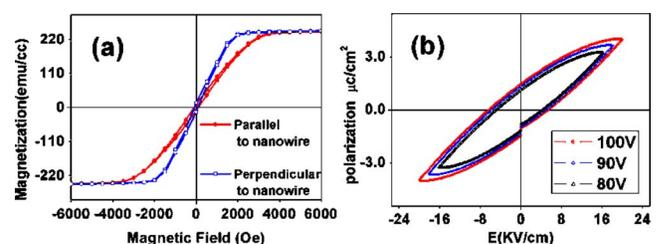
FIG. 5. (Color online) (a) Typical magnetic hysteresis loop for  $\text{NiFe}_2\text{O}_4$ -PZT core-shell nanowire arrays; (b) polarization-electric field hysteresis loops of the  $\text{NiFe}_2\text{O}_4$ -PZT core-shell nanowire arrays.
