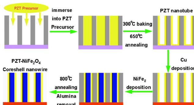
FIG. 1. (Color online) Schematic of the process flow for fabricating the ferrite core-PZT shell nanowire arrays.
