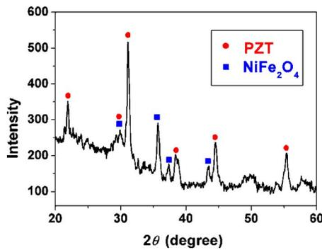
FIG. 2. (Color online) X-ray diffraction pattern of PZT- $\text{NiFe}_2\text{O}_4$  core-shell nanowire arrays in AAO template.
