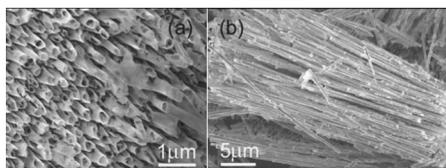
FIG. 3. SEM images of (a) open ends of PZT nanotubes with AAO template removed and (b) core-shell PZT- $\text{NiFe}_2\text{O}_4$  nanowires released from AAO template.
