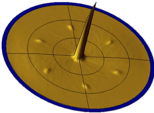
FIG. 3. (Color online) Pole figure obtained for a fixed value of  $2\theta=23.03^\circ$ . The single dominant peak corresponding to  $\phi=\psi=0^\circ$  corresponds to the  $\langle 006 \rangle$  reflection indicating low  $c$ -axis dispersion. The weaker peaks exhibiting sixfold symmetry correspond to the closely spaced  $\langle 104 \rangle$ -type reflections illustrating the epitaxial relationship between the BaM and the MgO buffer layer.
