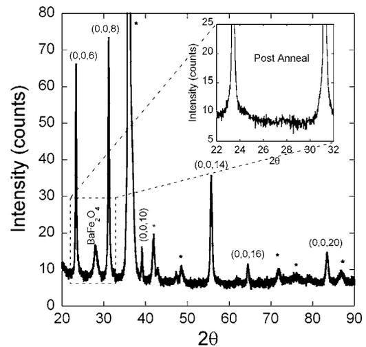
FIG. 2. X-ray diffraction pattern for Ba-hexaferrite ( $M$ -type) film. All significant diffraction features are referenced to  $(0,0,2n)$  indices having a space group of  $P6/mmc$ . The single  $\text{BaFe}_2\text{O}_4$  peak appearing near  $2\theta \sim 27^\circ$  disappeared after a postdeposition annealing procedure (see inset). (\* denotes SiC substrate peaks.)
