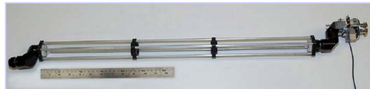
Figure 5. Existing articulated relay telescope that was developed by Gustavo Herrera for his master's thesis in the ECE Department and is now being further developed at Memorial Sloan-Kettering Cancer Center for imaging humans. The relay telescope couples at the galvanometric scanning mirror in Figure 1, and the endoscope will couple to this telescope to create an opto-mechanical probe interface to the human subject.
