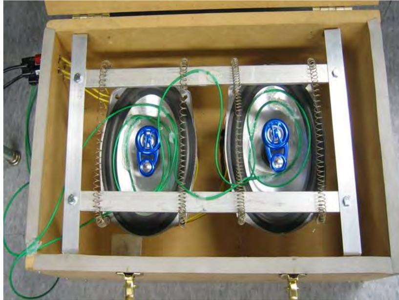
**Figure 10: Mechanical Dithering**
