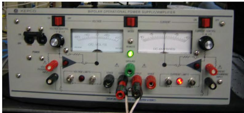
**Figure 16: Kepco BOP 20-10M Bi-polar Power Supply**
