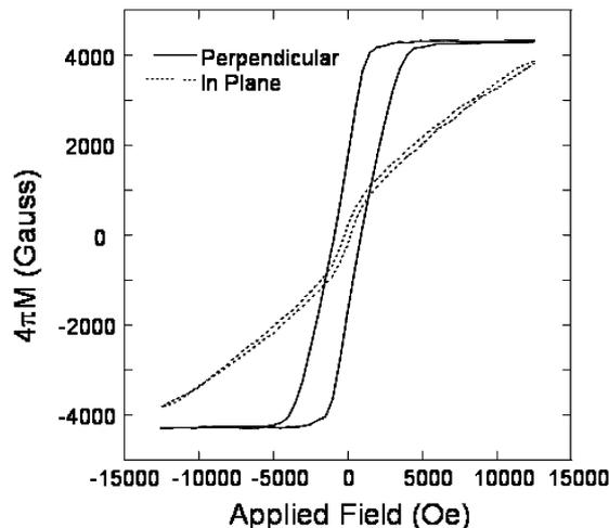
Fig. 3. Hysteresis loop obtained by vibrating sample magnetometry with maximum applied field of 12 500 Oe aligned parallel (dashed) and perpendicular (solid) to film plane. Data have not been corrected for demagnetization.
