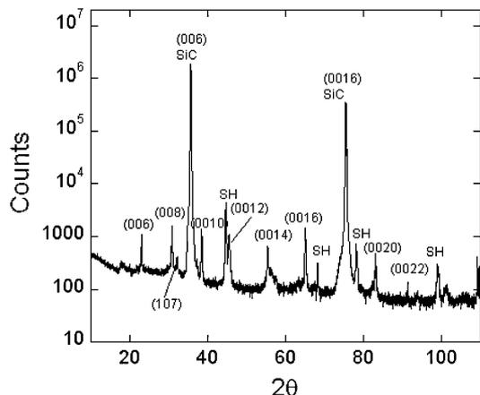
Fig. 1. X-ray  $\theta - 2\theta$  diffraction pattern for Ba-hexaferrite (M-type) film. All significant diffraction features are referenced to  $(0,0,2n)$  indexes having space group  $P6/mmc$  (SH denotes substrate holder).
