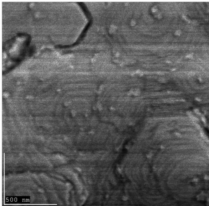
Fig. 2. AFM image processed in tapping mode illustrating hexagonal crystals oriented with  $c$  axis perpendicular to film plane.
